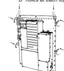
Fasten backplate screws (3/8 in screws, not supplied)
