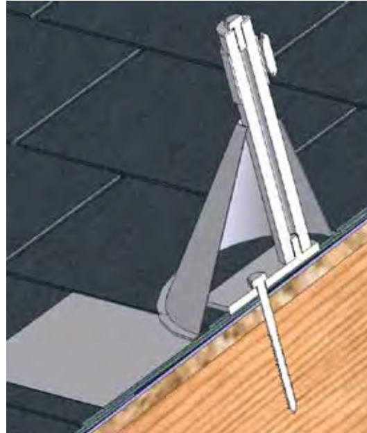
Fig 4.0 - Standoff section view
