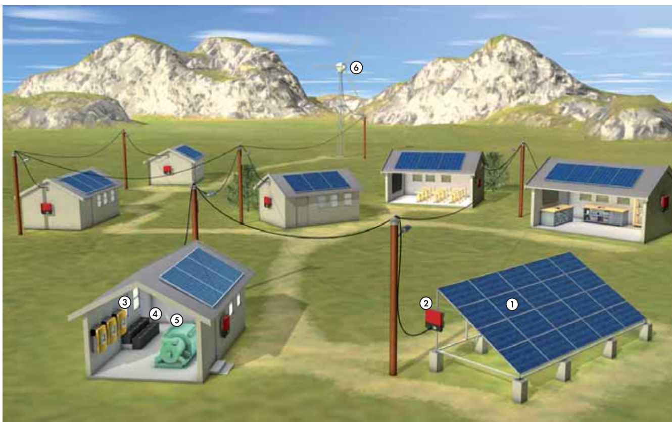
Components: 1. PV array, 2. SUNNY BOY, 3. SUNNY ISLAND, 4. Batteries, 5. Diesel generator, 6. Wind turbine system
