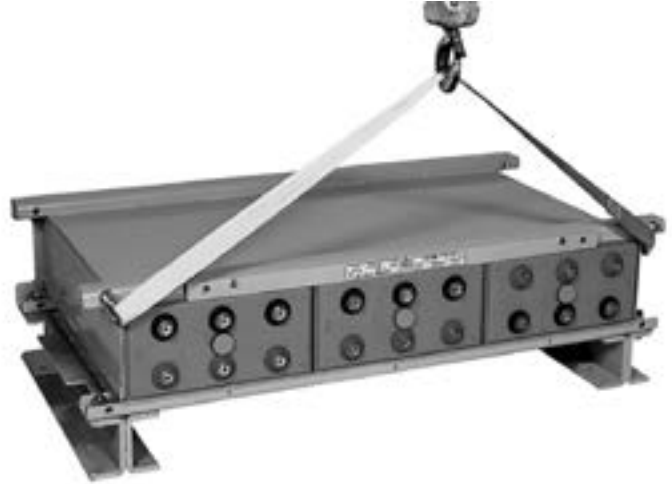
MODULE WITH BASE ASSEMBLY AFTER TIP-OVER Figure 13
