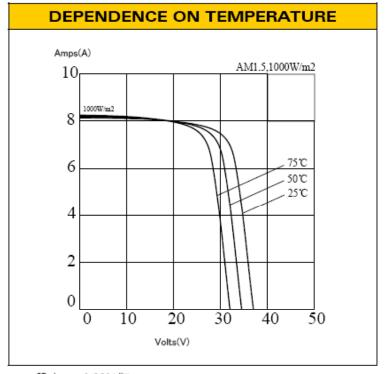
Temperature coefficient of Isc: 0.08%/°C
