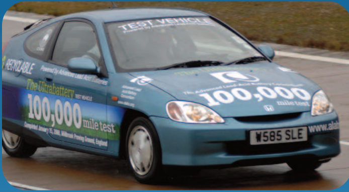
Figure 1. Shows the UltraBattery test vehicle when it went over 100K miles without a conditioning charge on January 15, 2008. The UltraBattery demonstrated better cycle life performance than the replaced Ni-MH battery pack.
