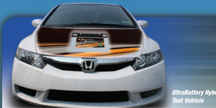
Figure 1. Shows the UltraBattery test vehicle when it went over 100K miles without a conditioning charge on January 15, 2008. The UltraBattery demonstrated better cycle life performance than the replaced Ni-MH battery pack.
