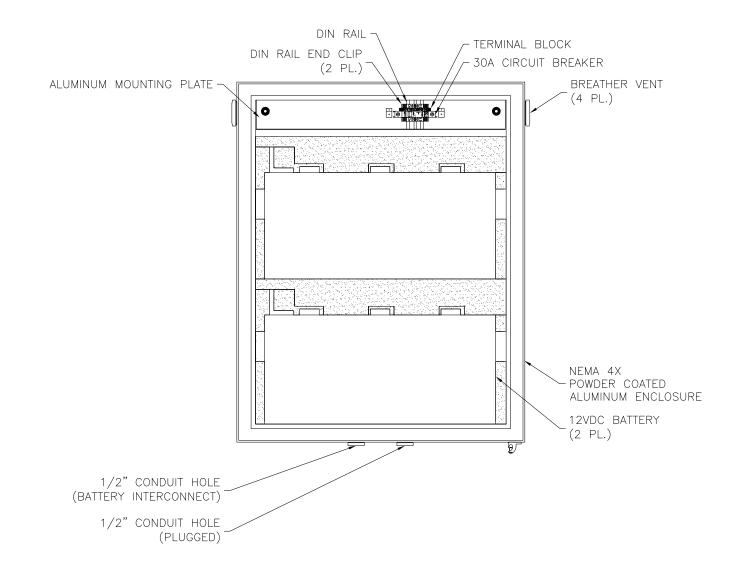
BATTERY TO HAVE EXPANDED POLYSTYRENE FOAM INSULATION ON ALL SIDES AND DOOR.
