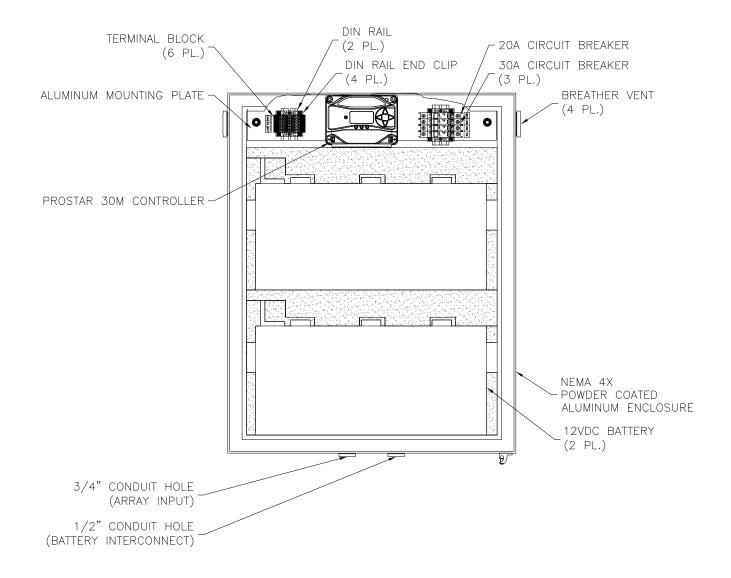
2. BATTERY TO HAVE EXPANDED POLYSTYRENE FOAM INSULATION ON ALL SIDES AND DOOR.
