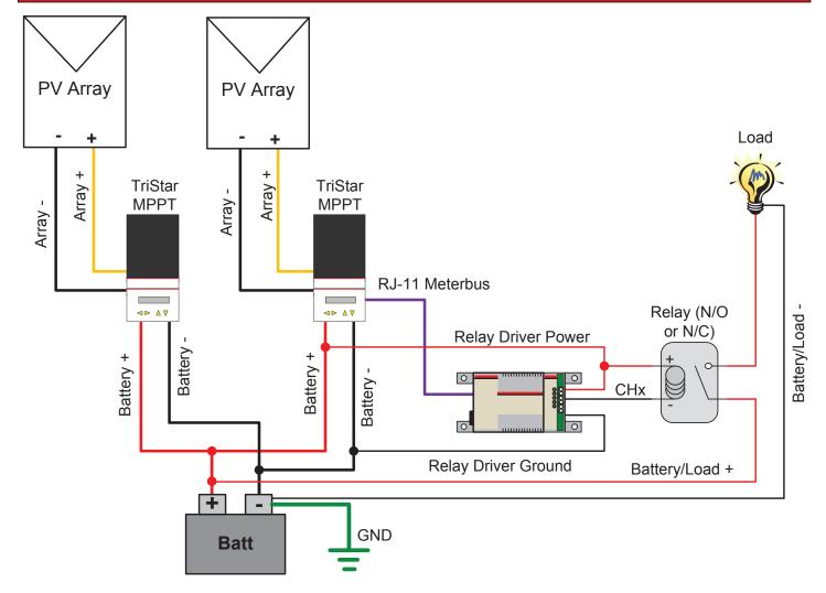
**IMPORTANT:** This is not intended to be a complete system diagram; fusing, disconnects, and grounding should comply with local electric codes.
